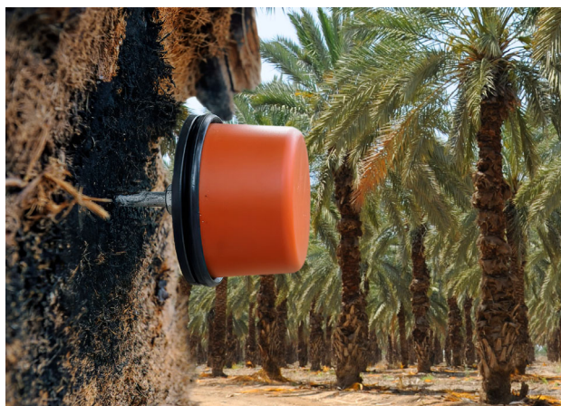
Figure 1. Agrint IoTTree seismic sensor installed in a date palm in Ein Yahav, Israel.
